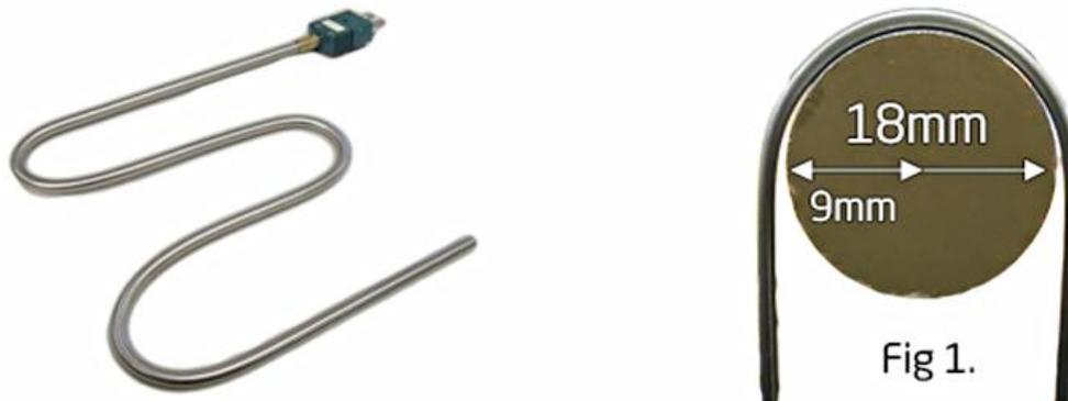
Mineral Insulated Thermocouples can be bent in to many elaborate shapes. However, there is a minimum bend radius, which is 3 times the cable diameter.
