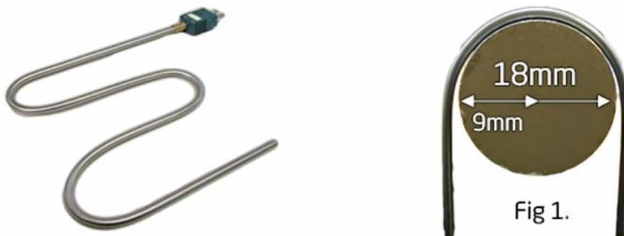
The above image shows a 3mm diameter MI cable at its minimum bend. To calculate the minimum bend radius you simply multiply the diameter of the cable by 3, therefore the minimum inside radius of a bend for 3mm cable must be  $3 \times 3 = 9\text{mm}$ .
