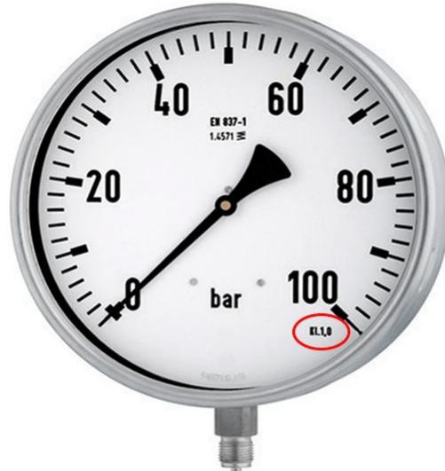
The accuracy class is shown on the dial as Acc, Class, CI or KI (e.g. **CI 1.0 for 1% of full scale value**).
